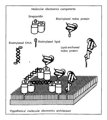
Fig. 1. Illustration of molecular electronics components and potential architectural features of self-assembling systems restricted to diffusion in two-dimensional lipid films.
